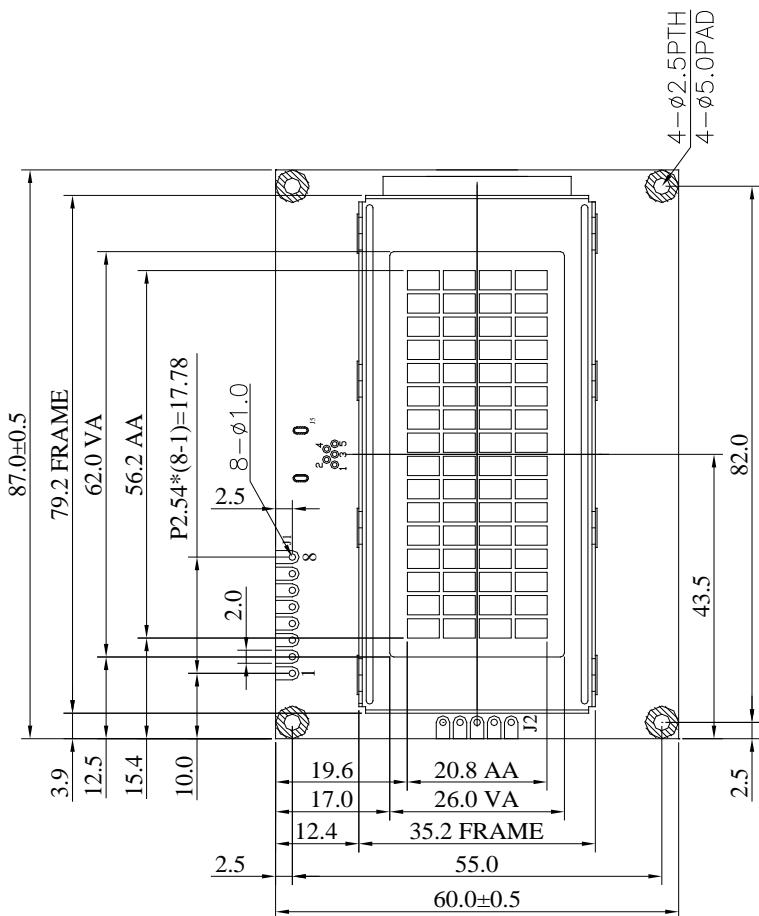
THE NON-SPECIFIED TOLERANCE OF DIMENSION IS  $\pm 0.3$ mm
